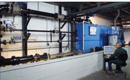
We test our valves under actual process conditions in our advanced flow lab to ensure our solutions perform as promised in your application.
