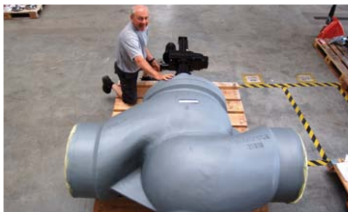
DN600: Erwin Hintke will conduct the tests for this direct-flow control valve.
