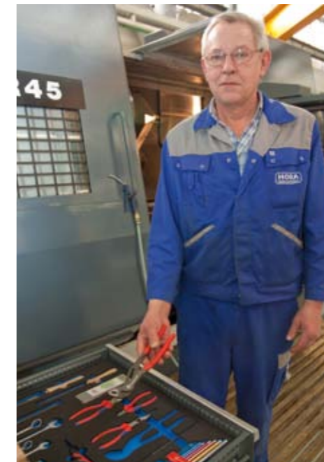
Werner Schnitker (left) with the checklist. Manfred Krypczyk shows his drawer arrangement at the 5S reference workstation. The blue mark indicates a missing tool.
