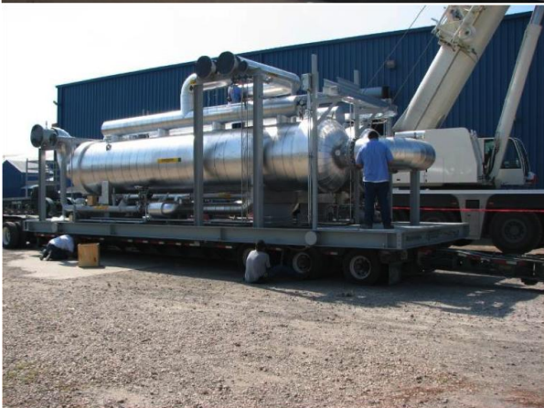
Above top left: modular assembly produced on the shop floor; Left: ORC skid being loaded onto a truck for transportation to a project site; Above: a 4MW waste heat installation on an existing dual-turbine gas compression site (the ORC system and its heat rejection is circled in red)
