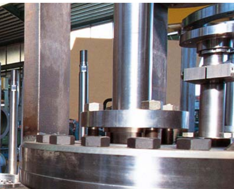
The assembly and testing of industrial valves, that weigh tons calls for millimetre precision and finger-tip feeling – as in these eight turbine bypass valves for a power plant in India. Complicated function tests and final approval testing over several days face the assembly personnel with ever new challenge.
