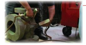
Magnetic Particle Test.- In a random basis for standard products or when a Customer request MT Certification, WALWORTH has the Magnetic Particle Test Equipment to perform on Ferrous materials susceptible to magnetism.
