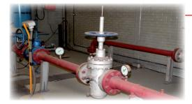
**Test Loop**.- A complete Laboratory Test loop exists for design validation of **WALWORTH** products performing the test at maximum design pressure and cycling the valves from 3000 to 5000 cycles. The test expends more than 4 months to be finished.
