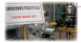
**Low Fugitive Emissions Test.-** When a Customer requires low fugitive emissions certification, The Lab has its own LFE Test Equipment capable to measure less than 20 ppm either in both static or Mechanical conditions at ambient temperature or thermal cycle operations.
