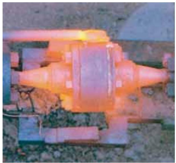
**V&W fire safe ball valves have been successfully tested accordind to BS 6755, API 607, and API 6FA Fire test procedures.**
