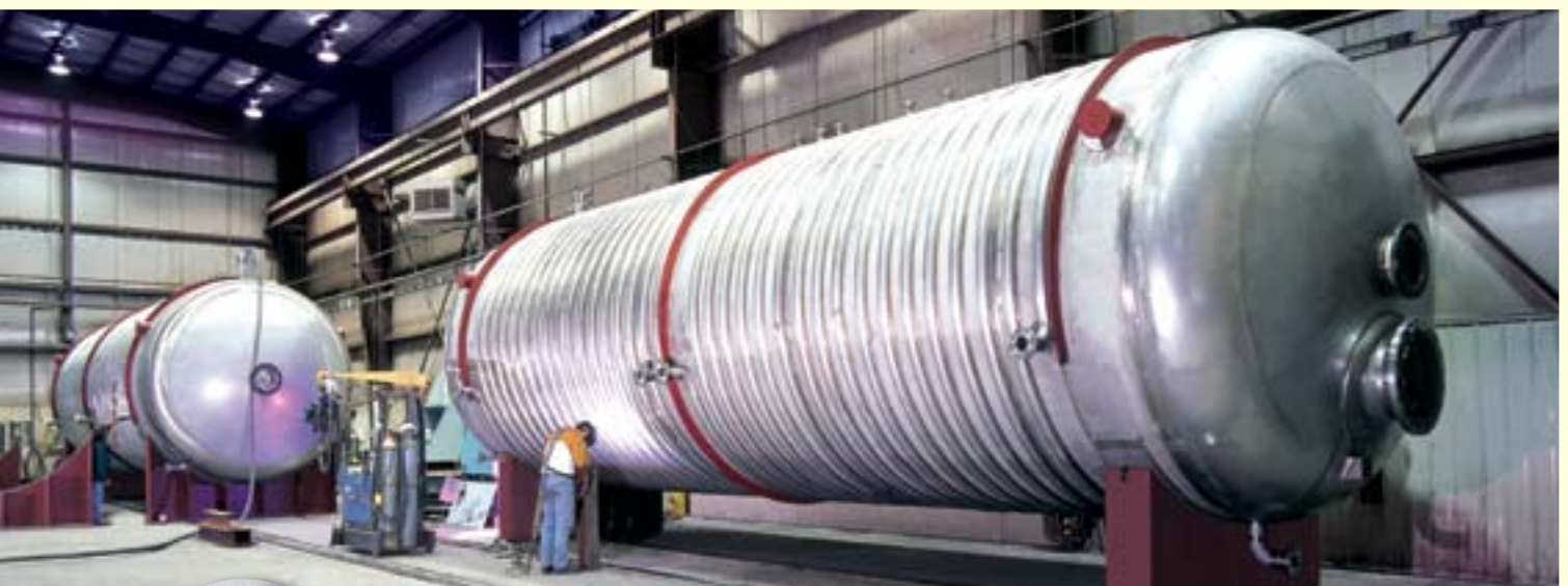
Horizontal Storage (Lethal Service) Tanks 30,000 Gal Each
