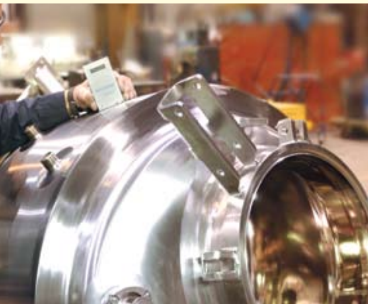
Ra Test to Confirm Surface Finish Compliance
