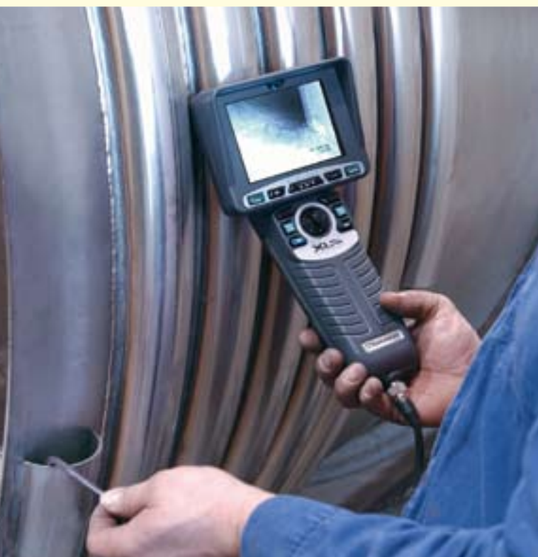
BoreScope to View Internal Welds
