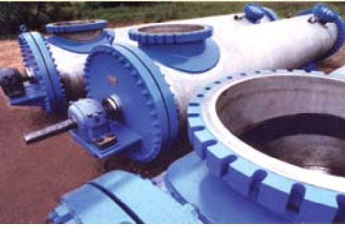
45" Dia. x 20' Long Digester Tubes
