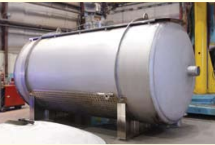
Horizontal WFI Surge Tank
