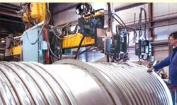
Installation of 165° Half Pipe with Guaranteed 100% Weld Penetration
