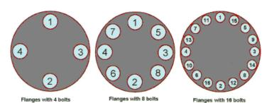
VI. Bolts should now be torqued 45% to 65% of the bolts yield value in a four (4) step tightening sequence. Torque figures are determined by the bolt diameter, the material from which the bolts are made and in service temperature should be considered at times. Sealing Corporation recommends the use of B-7 Bolts or equivalent whenever feasible.
